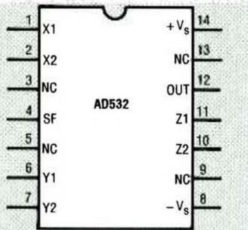
FIG. 10—PINOUT DIAGRAM for an AD532 in a 14-pin DIP.
