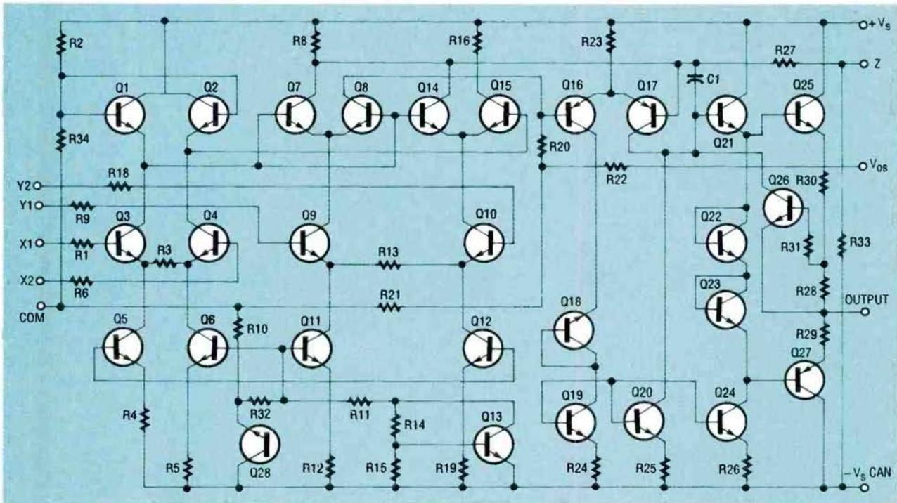
FIG. 9—SCHEMATIC DIAGRAM for a monolithic AD 532 multiplier.
