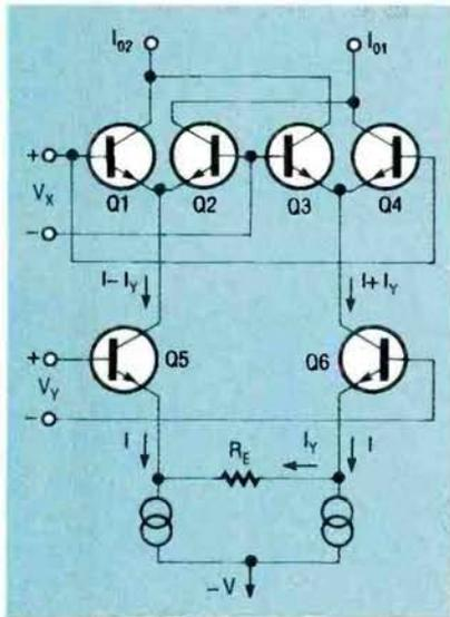
FIG. 7—FOUR-QUADRANT MONOLITHIC modulator is basically two two-quadrant transconductance multipliers.
