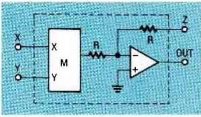
FIG. 1—FUNCTIONAL BLOCK DIAGRAM of a typical multiplier/divider.
