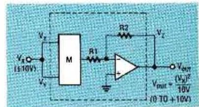
FIG. 5—MULTIPLIER IC CONNECTED as a squarer.
